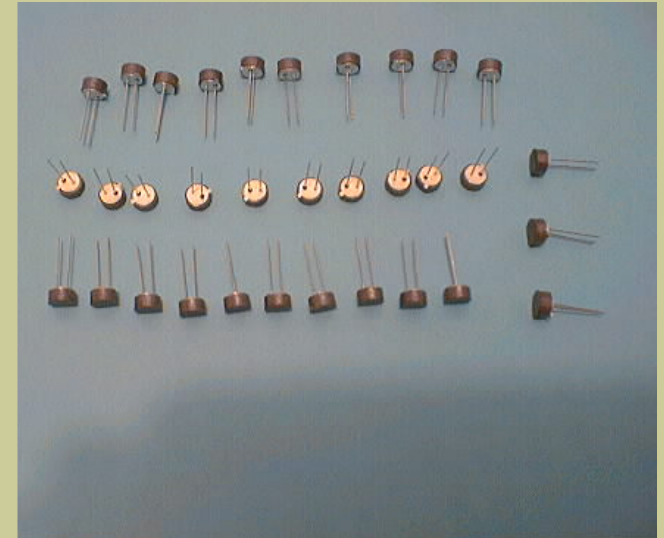
Mounted shields on portion of 90 TO metal cans
